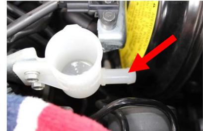
13) Next with the packing still under/around the master cylinder use a 10mm Flare Nut Wrench remove the factory hard line from the right side of the master cylinder. (Note: paper towel packing has been removed for photo clarity)
