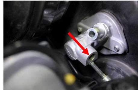
14) Locate the brass junction point in the fender well and remove the **Upper** hard line using a 10mm Flare Nut Wrench (Tip- Use shop towels underneath the fitting to catch any fluid that leaks). **Do Not Disconnect the Lower Line running to the transmission.**
