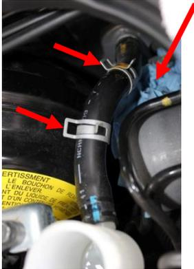
10) Using pliers squeeze the tabs on the reservoir line clamps to release them and move them towards the center of the line.
