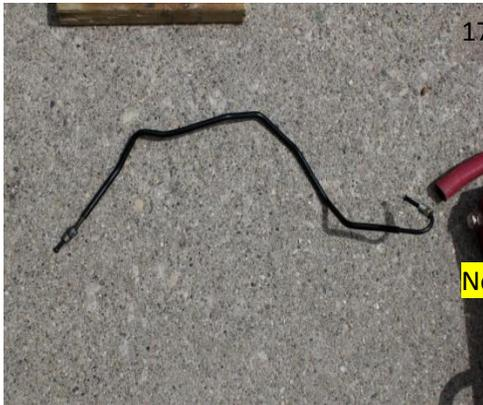
17.) 17.) With the master cylinder out you can carefully pull the upper hard line up and out of the car from the top side where the master cylinder is. Pull the line carefully up thru the frame and work it carefully out. It may take a bit to work all the kinks/bends thru the frame but it should come out fairly easily. A little bending or flexing of the line may be required to get past certain points which is perfectly OK, just be gentle and don't kink or cut the tube getting it out.
