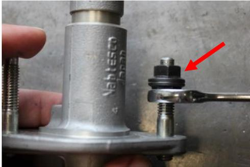
**(follow instructions with the tool) or two of the master cylinder nuts using the following procedure:**
