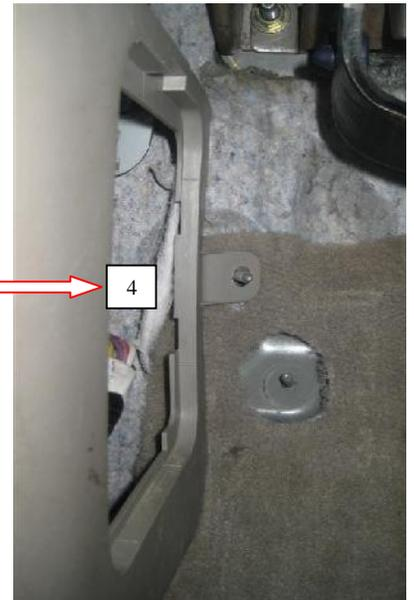
4.) Remove the small hatch cover in the center of the kicker panel to get a better grip and start gently pulling the panel outwards. Work from the top corner closest to you along the door edge and the clips will start popping free. Once you've worked down the edge you can pull the panel out and set it outside the car along with the center hatch.
