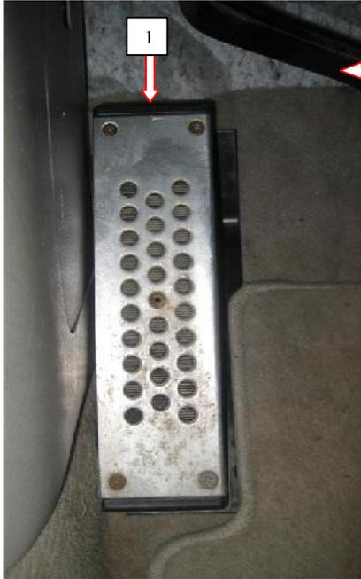
1.) Start by removing the dead pedal. To do this grab in the top center and pull towards yourself. The clip will disengage from the floor. Next grab the bottom and pull it up as well. If you see round black plastic pieces sticking up from the floor then spin these off the little studs welded to the floor and snap them back into the holes in the bottom of the dead pedal.
