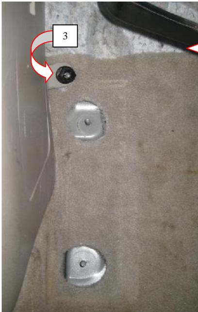
3.) Next Remove the Black Plastic Nut holding the corner tab of the LH Kicker Panel to the floor using your fingers or some pliers to get it started.
