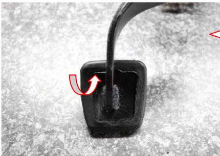
16.) Next carefully pull the pedal cover from the factory pedal starting at the top left corner by rolling the rubber lip back out of the way and pulling the cover off.
