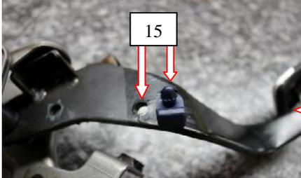
15.) Use pliers to squeeze the back of the blue stop bumper and push it out of its hole in the factory pedal arm.
