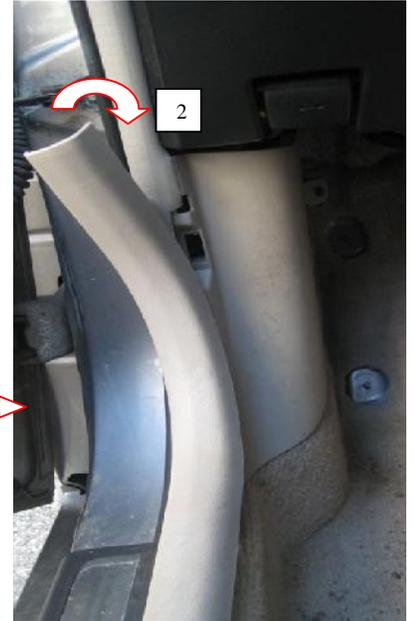
2.) Now gently pull up the Door Sill Trim starting at the front where it meets the dash Panel. Just work this up a little at a time and the clips will release.
