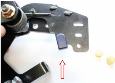
18.) Take the Blue Stop bumper and press it thru the hole on the new pedal arm as shown so the flat face is on the Left Side.
