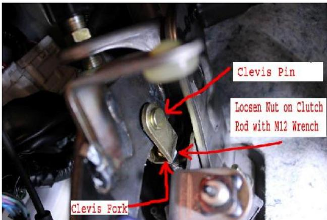
7.) Use an M12 Wrench to loosen the clutch rod nut located behind the clevis fork (Seen in photo below)
