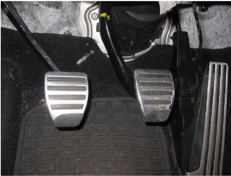
41.) With the AFP Adjuster set to roughly around 70% (doesn't need to be exact) and the return spring still sitting loose have a look at how high the new clutch pedal is relative to the brake pedal height. Using your Needle nose pliers turn the clutch rod Right (Counter Clockwise) until the clutch pedal is leveled up with the brake pedal height while leaving the 2pc arm adjustment centered.
