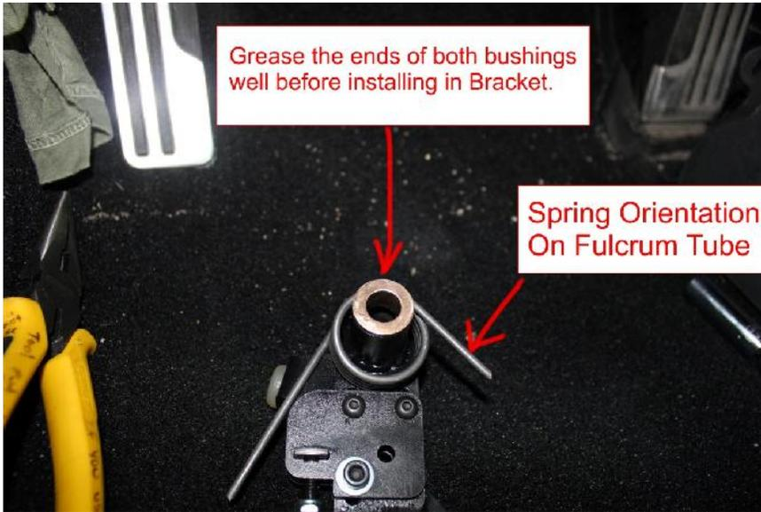
33.) Next take the spring and place it over the RH side of the pedal arm pivot tube. Don't clip it into its keeper yet. Leave it floating loose with the long side pointing somewhat upwards.
