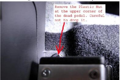
1.) Remove the black plastic thumb nut above the dead pedal which holds the LH Trim Panel.
