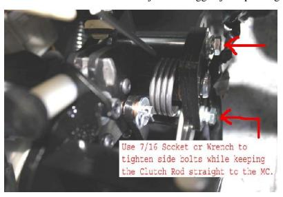
36.) Now check the pedal arm for free side to side play. If the pedal can still rock slightly side to side then tighten the two side bolts evenly a ¼ turn at a time until you feel the side play just disappears and no more. This sets the side-load on the fulcrum shaft bearings and if over tightened will cause the pedal arm to become stiff and bind up the bearings.
