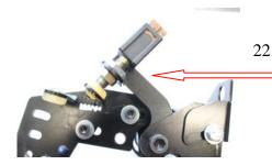
22.) Next install the Brown Cruise Control switch into the upper switch mount followed by an oem switch lock nut. Set this switch so there is an equal amount of threading on either side of the metal tab and tighten both lock nuts using your 14mm & 17mm wrenches together.
