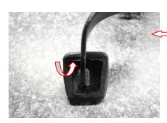
16.) Next carefully pull the pedal cover from the factory pedal starting at the top left corner by rolling the rubber lip back out of the way and pulling the cover off.
