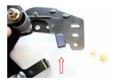
18.) Take the Blue Stop bumper and press it thru the hole on the new pedal arm as shown so the flat face is on the Left Side.
