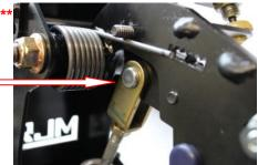
29.) Now get a Deep 12mm socket, long extension and ratchet ready for this step. Moving the bracket up or down alters the angle of the clutch rod which needs to push straight in/out of the master cylinder. Move the bracket to where the rod looks to be going straight into the master cylinder and tighten the upper right stud nut firmly, followed by tightening the lower left stud nut firmly and finish by tightening the upper dash bolt. (See Reference Photos at Steps 26 & 27)
