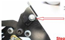
30.) Use a 7/16 wrench or socket on your ratchet and tighten the upper right cross bolt that clamps the upper dash mount to the main bracket. This only needs to be snugged up + half turn. Don't crank this down overly tight or it could start to collapse the main bracket or strip the threaded nut on the other side. (Shown out of the car for clarity)
