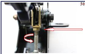
31.) Use a 12mm wrench and loosen the lock nut on the clutch rod, behind the clevis fork.
