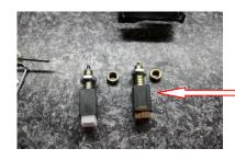
20.) Spin the factory lock nut off both switches and swap them for the larger lock nuts supplied in the kit.
